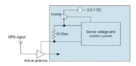
Antenna Detection Circuit
