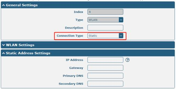
R1520 does not support "PPPoE" WLAN connection types.
