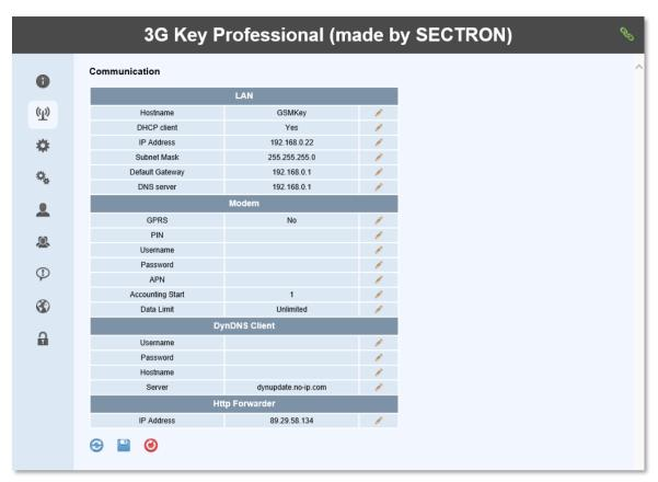
Parameters for connection via an Ethernet cable.
