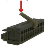
In the event the hook gets lost, it is possible to use a thin flat 2mm screwdriver, which is inserted into the upper hole. Gently push inwards until the wiring lock opens. In the case of a small opening, it is possible to open the lock up more by gently lifting up the screwdriver.
