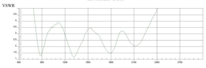
Frequency(600 - 3000 MHz) Resolution: 521 Cal: ON
