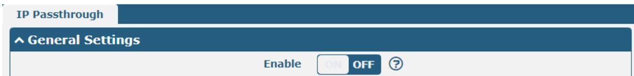
When the router turns on the IP Passthrough function, the terminal device (such as a PC) will open the DHCP Client mode and then connect to the LAN port of the router. After the router successfully dials the number, the PC will automatically obtain the IP address and DNS server address assigned by the operator.
