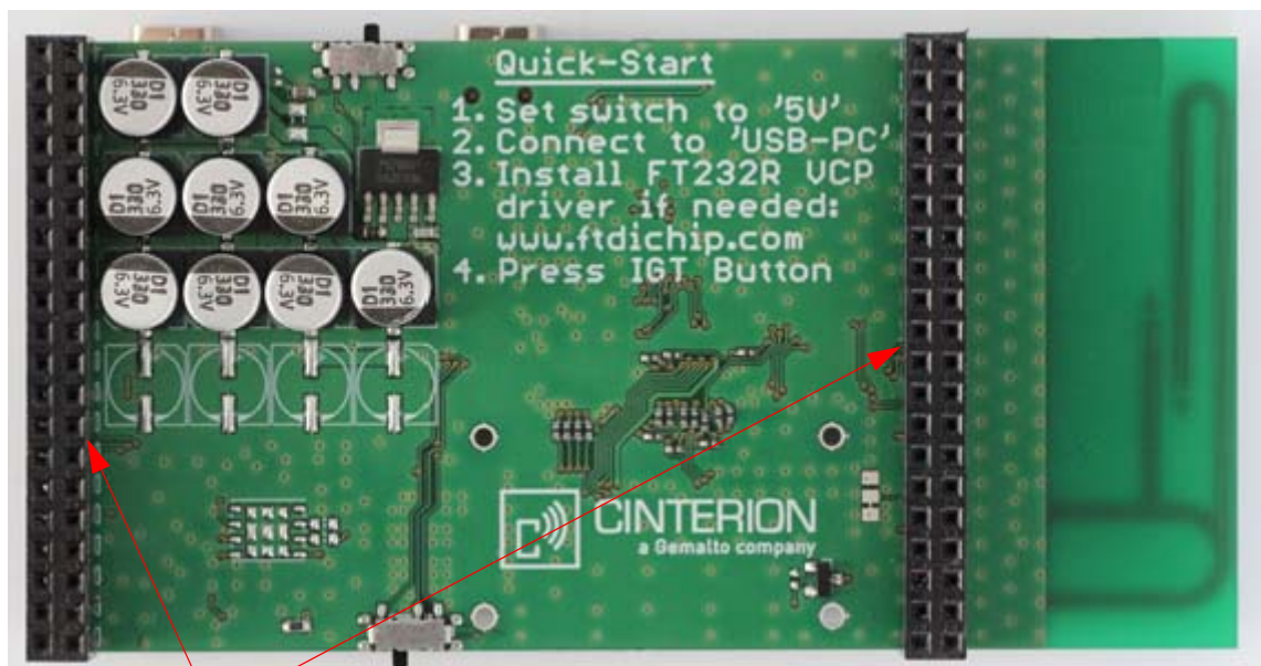
2x40-pin connector for access to the module's interface lines including power supply
