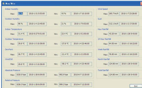
This section is used to display the recorded min and max value recorded with time stamp. Min/Max reset can only be done through key operation on the base station.
